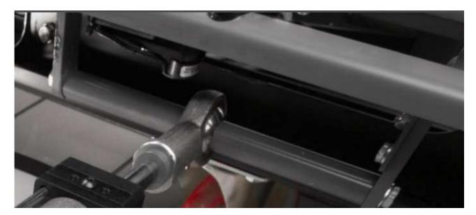
On the other side of damper complex there is a bracket with 4 holes with 40mm distance, fixed with 4 M6 bolts.
